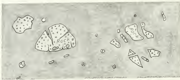
Fig. 6.—Character of ore at Creighton mine, Sudbury area, Ontario, ninth level, 15 feet from footwall. Greenstone boulders and fragments enclosed in sulphides (shaded area). Width of face 8 feet.
